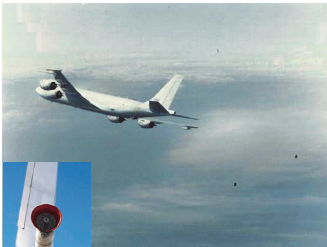
Figure 20 - TAC IVB HPTS E6B in Flight with Drogues Coming Out (Rear Drogue Inset)
